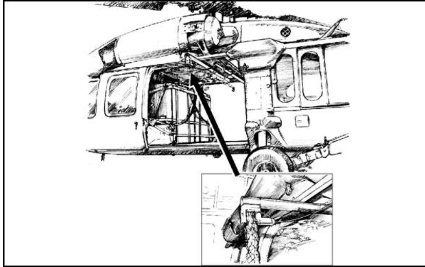
Figure 5-2. Bar assembly correctly mounted to aircraft.
